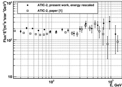
Figure 1: Comparison of the electron spectrum of ATIC-2 of present paper with the spectrum of the paper [1]. The proton background is not subtracted in both spectra.
