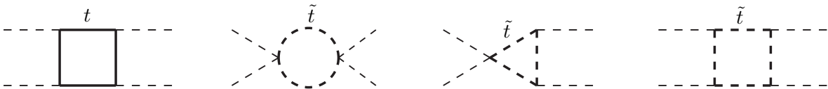
Figure 8.3: Integrating out the top quark and top squarks yields large positive contributions to the quartic Higgs coupling in the low-energy effective theory, especially from these one-loop diagrams.
