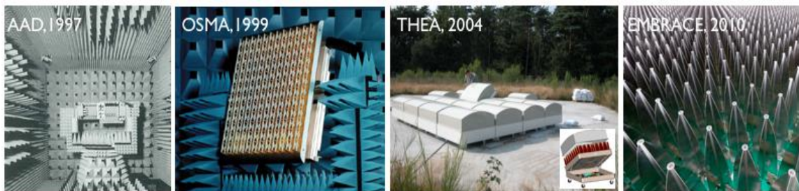
Fig.1 Some of the engineering test systems that have advanced the development of Aperture Array technology for radio astronomy under the leadership of ASTRON [9].
