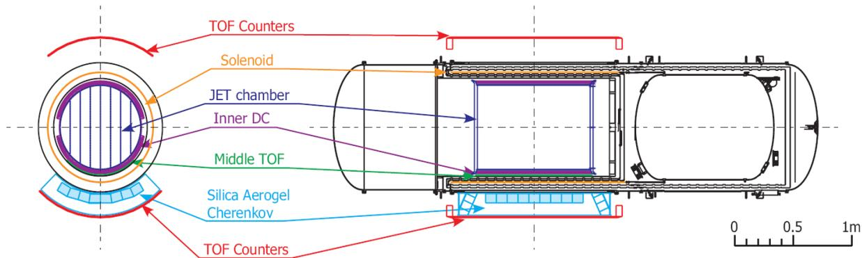
Figure 1: The cross-sectional view and the side view of the BESS-Polar II Spectrometer.
