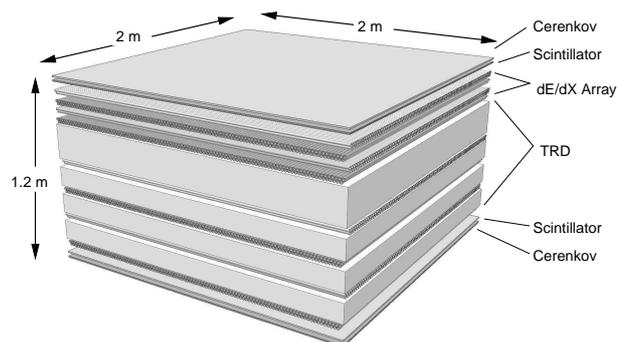
Figure 1: Schematic view of the detector elements of TRACER.
