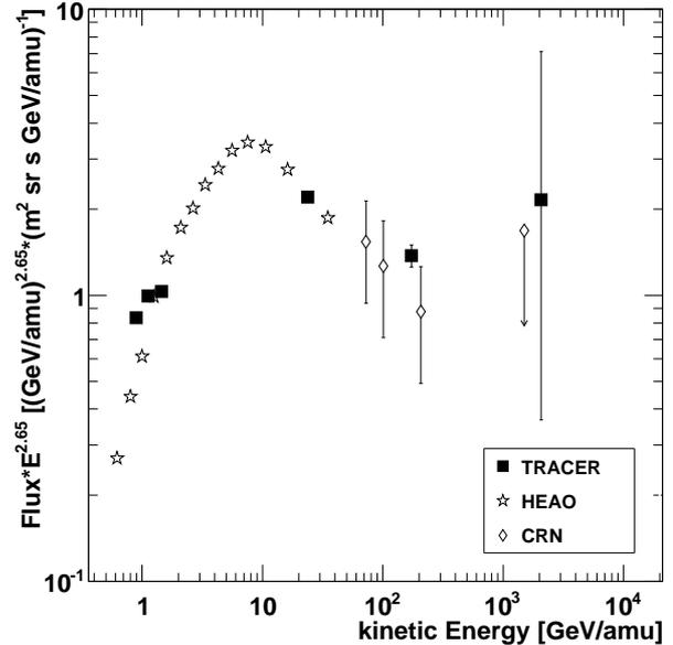
Figure 5: Differential energy spectrum of boron. The spectrum is multiplied by  $E^{2.65}$ . For comparison, results from HEAO [4] and CRN [12] are shown. The error bars are statistical.
