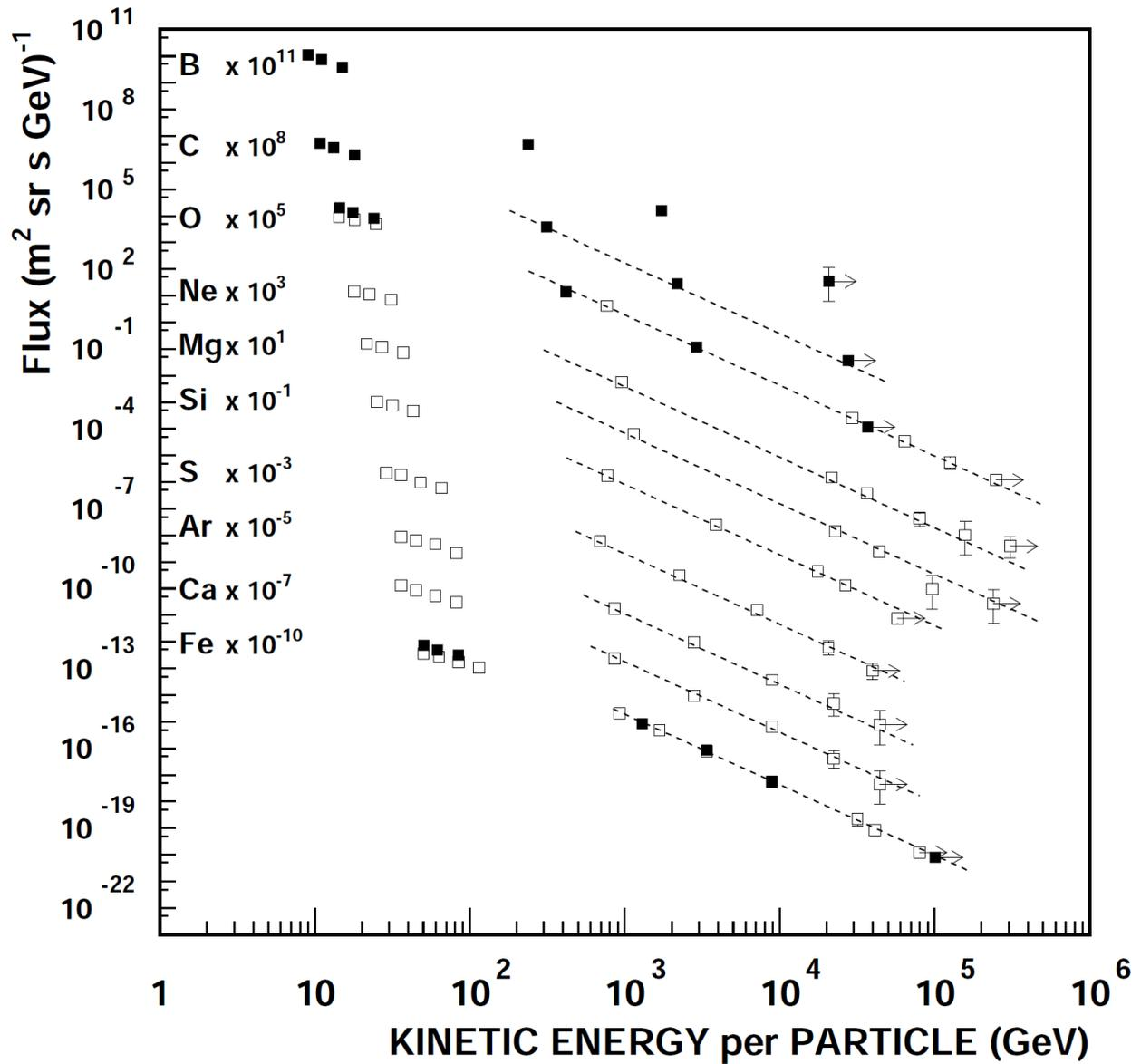
Figure 6: Compilation of the differential energy spectra measured by TRACER in LDB1 [2] (open symbols) and LDB2 [8] (filled symbols).
