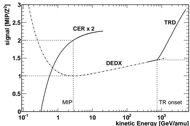
Figure 3: Response functions, in units of signal at minimum ionizing energy (MIP) normalized by  $Z^2$ , of sub-detectors used for energy measurements. The dashed lines indicate the signals at minimum ionizing energy and TR onset.
