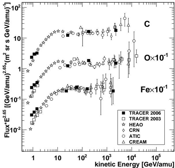
Figure 4: Differential energy spectra of carbon, oxygen, and iron (top to bottom). The spectra are multiplied by  $E^{2.65}$ , as well as divided by 10 for oxygen and iron. For comparison, results from HEAO [4], CRN [6], ATIC [11], and CREAM [1] are shown. The error bars are statistical.
