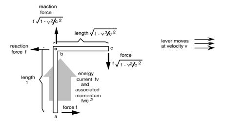
Figure 2: Lewis and Tolman's Bent Lever Showing Reaction Forces and Effects of Motion
