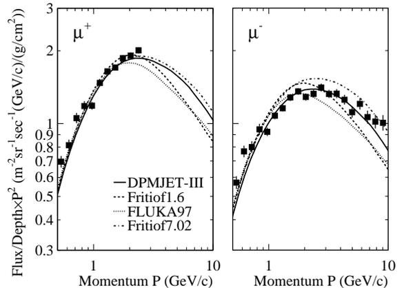
Figure 4. Observed and calculated  $[Flux/Depth]$  of muons at small atmospheric depth.
