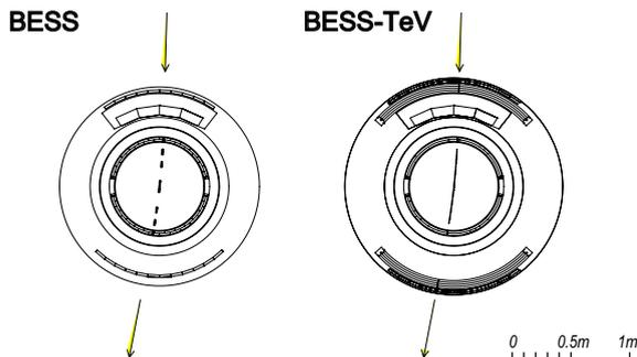
Figure 1. Schematic cross-sectional views of BESS and BESS-TeV spectrometer.
