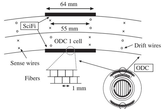
Fig. 2. Schematic view of SciFi mounted on ODC.
