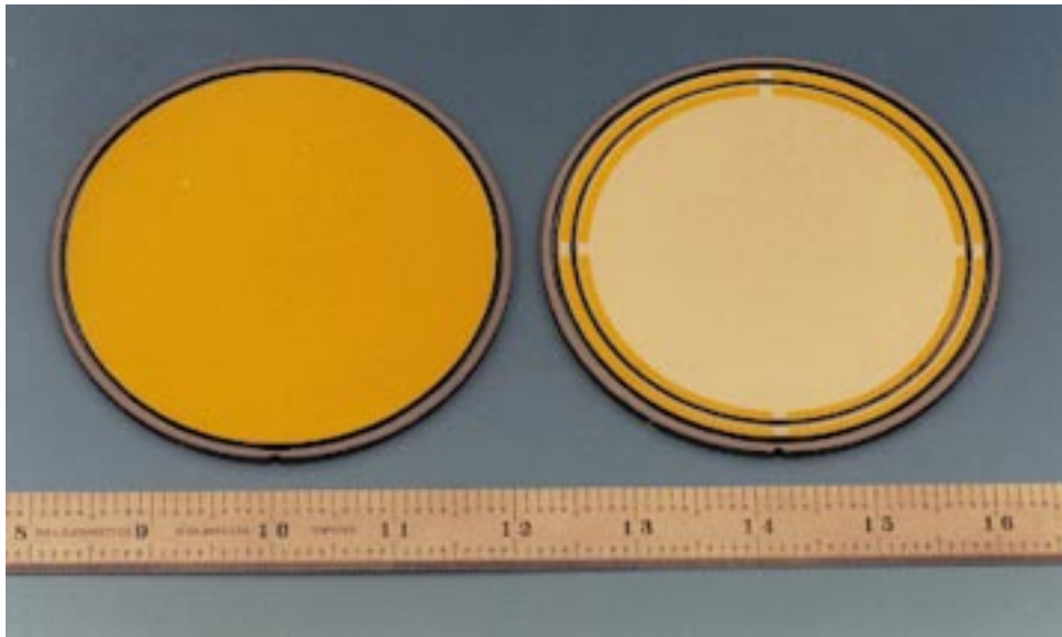
Figure 10. Photographs of CRIS stack detectors. A single groove detector is on the left, and a double groove is on the right. The silicon wafers are 10 cm in diameter and 3 mm thick. The annular region between grooves of the double-groove detector serves as an active guard region for identifying particles which exit or enter through the sides of the stack.
