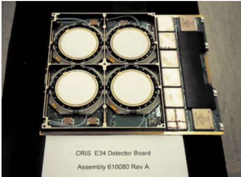
Figure 17. Photograph of a CRIS detector board with all parts installed. The four detectors are surrounded by conducting ‘fences’ which serve as RF shielding and have precisely machined heights that permit stacking of successive detector boards with minimal build-up of tolerances. Immediately to the right of the detectors are eight hybrid pulse-height analyzers: on this board they process signals from E3AB, E4AB, E3CD, E4CD, G3AB, G4AB, G3CD, and G4CD.
