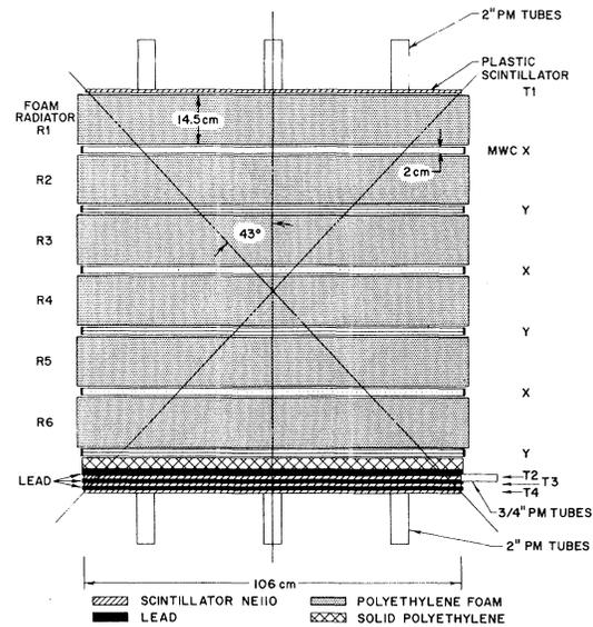
FIG. 1. Schematic cross section of the instrument.
