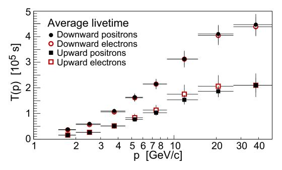
Figure 6: The livetimes, averaged over the detector acceptance, as functions of momentum for downward (circles) and upward (squares) going positrons (filled) and electrons (open).
