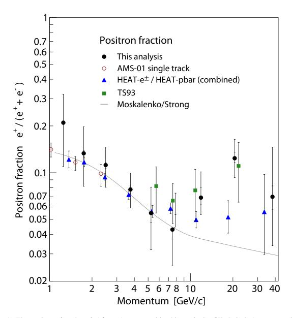
Figure 4: The positron fraction  $e^+/(e^+ + e^-)$  measured in this analysis (filled circles), compared with earlier results from AMS-01 (open circles) [12], TS93 (squares) [13], the combined results from HEAT- $e^\pm$  and HEAT-pbar (triangles) [14], together with a model calculation for purely secondary positron production from [15] (solid line). The total error is given by the outer error bars, while the inner bars represent the systematic contribution to the total error.
