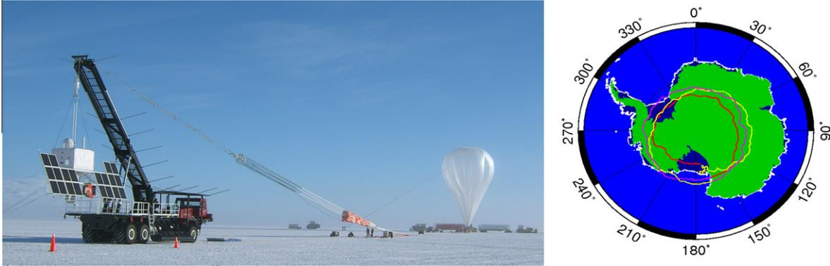
**Fig. 1.** (a) CREAM ballooncraft with the launch vehicle while a  $\sim 1$  MCM balloon is being inflated at the launch site, Williams field near McMurdo, Antarctica; (b) Balloon trajectory of a 37 day flight of CREAM, which was launched on December 1, 2009 and terminated on January 8, 2010 during about 3 rounds of the South Pole.
