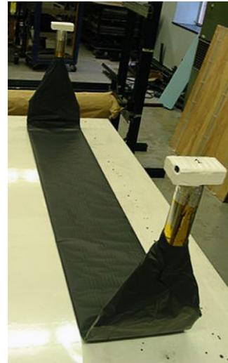
Fig. 4. Individual TCD paddle with potted PMT assemblies at its ends.
