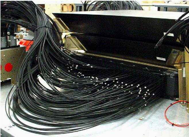
Fig. 10. Calorimeter mounted under graphite targets during assembly of the calorimeter module. Shown in the foreground are the IFO fiber bundles carrying light signals through light-tight wall to a readout box.
