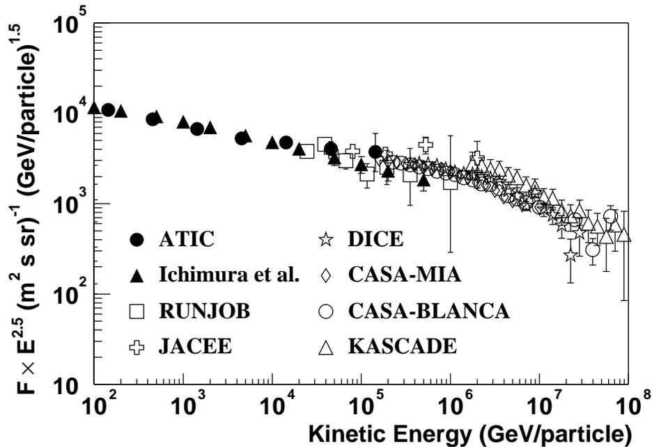
Figure 2: All-particle spectrum measured by ATIC (filled circles), together with those measured by other direct and indirect experiments, Ichimura et al., RUNJOB, JACEE, DICE, CASA-MIA, CASA-BLANCA, and KASCADE.
