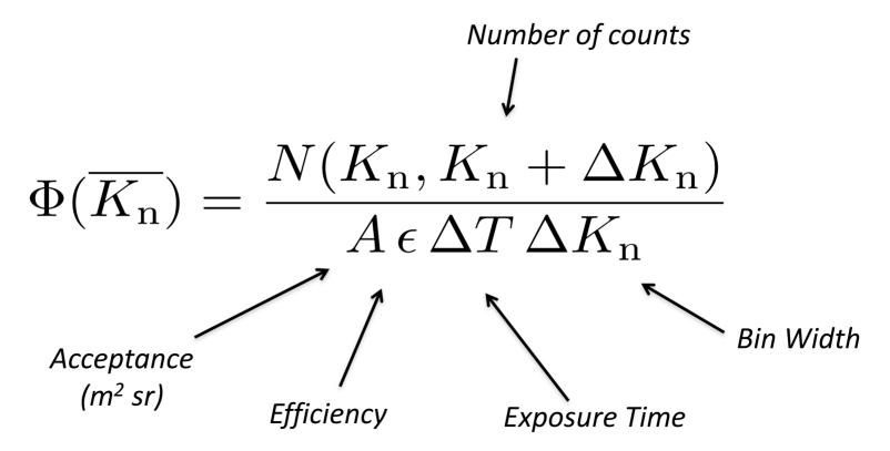
*K<sub>n</sub>* is the **kinetic energy per nucleon**, is measured from TOF and RICH (beta) or from Tracker (rigidity)
