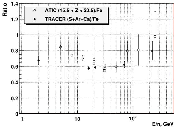
Figure 6: Comparison of the “almost direct” data of TRACER [11] for the ratio (S+Ar+Ca)/Fe with the data of ATIC for the ratio ( $16 \leq Z \leq 20$ )/Fe.
