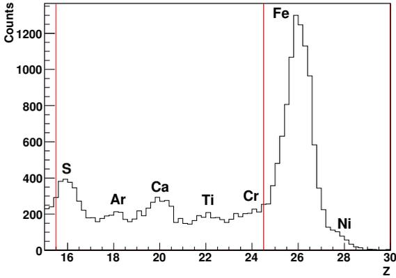
Figure 1: A fragment of charge spectrum as measured by ATIC spectrometer for  $E > 60$  GeV per particle. The charge region between two vertical red solid lines corresponds to  $H^-$  region (see the text).
